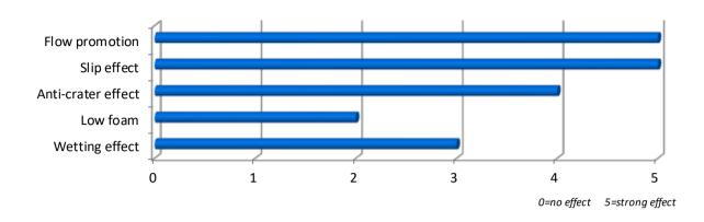
**UNIC**<sup>®</sup>**FLOW 477 U** is modified polyether polysiloxane leveling agents. The product can offer strong reduction of surface tension and improves wetting effect and anti-crater effect of substrate. Meanwhile, it shows the good performance of fast leveling with excellent hand feeling and slip effect.
